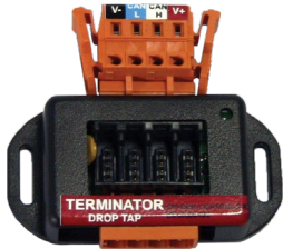
Fig. 1A: Terminator taps are located at each end of the network.
